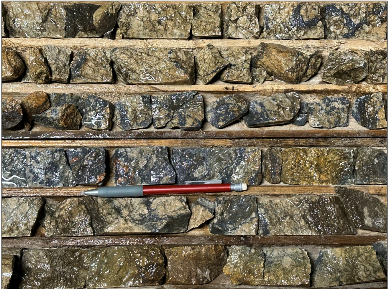
Figure 12-2: Close-up view of drill hole 324-03-1977 showing abundant galena within brecciated dolostone
