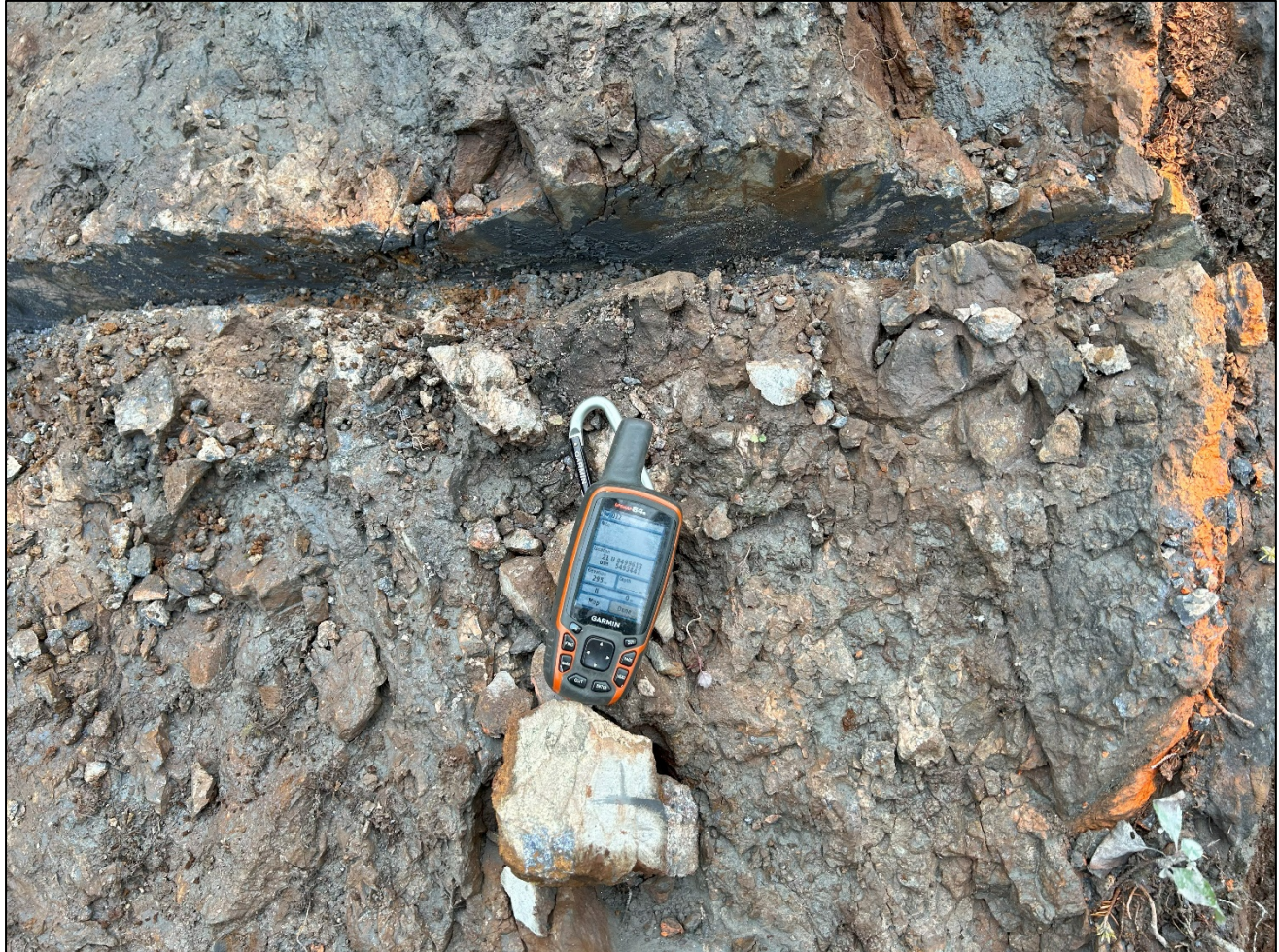
Figure 12-4: IW grab sample 3083 with massive galena (Pb) mineralization taken from Trench 23-01
