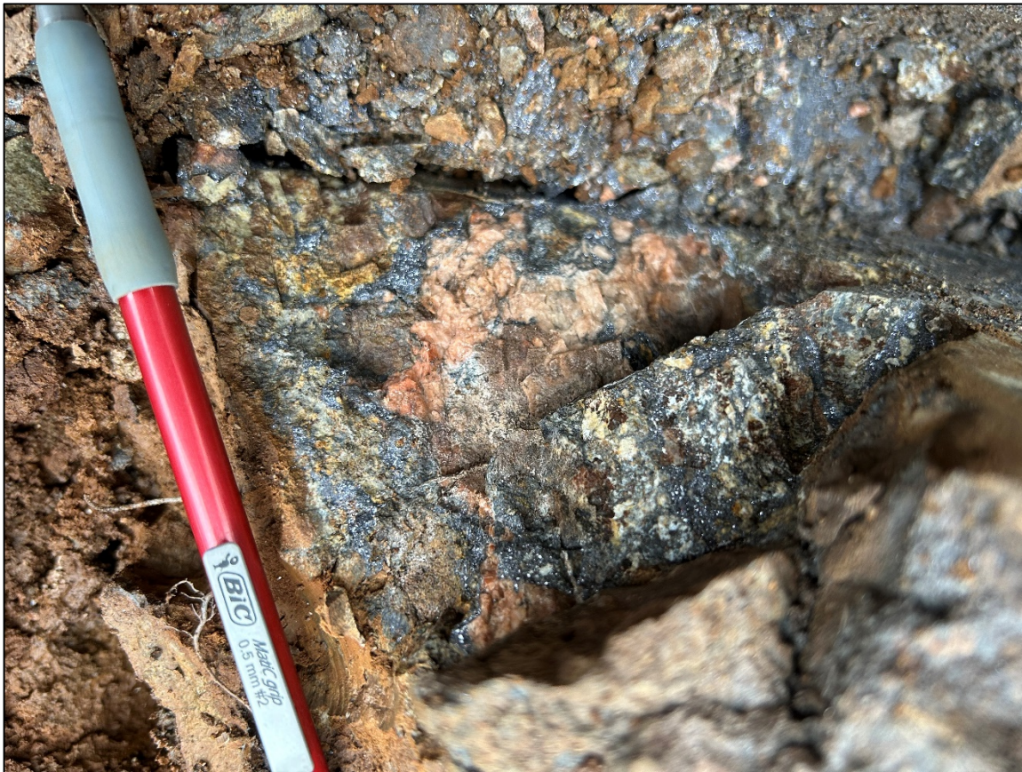
Figure 2-2: Close-up view of brecciated dolomitic limestone with massive galena (>20%)
