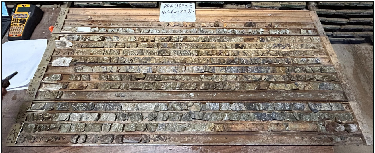
Figure 12-1: Brinex-Noranda drill hole 324-03-1977 with massive galena mineralization close to the surface
